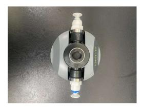
14. Now that the filter is fully installed, use a measuring container to verify that the water flow rate is 0.45 gallons (1.7 liters) per minute. If necessary, adjust the flow rate using the T-valve installed earlier. This will ensure optimal filtration performance.
